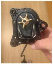
If there is excessive calcium in the water for example, which clogs the pump, the pump needs to be cleaned.
