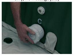
If the filter is mounted elsewhere, the water will not pass through the filter cartridge, which is supposed to catch mechanical impurities (hair, etc.), and will clog the pump outlet instead. Impurities that enter the filter system like this may damage it – pump jamming, scraping the pump duct, breaking the axle, etc. These types of damage are not covered by the warranty.
