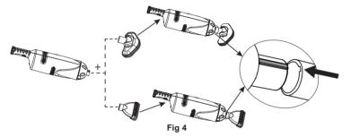
4. Attach the aluminum pole (9) by squeezing the spring buttons and inserting into handle of the vacuum body (1). Check the buttons "pop" into the holes. Adjust the length of the shaft by unlocking, extending and locking each section accordingly. See fig 5. Optional: The included pole adaptor (10) can be used with other sizes of extension poles.
