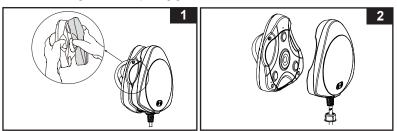
Place the transmitter (2) on the outside of the pool wall and the pool light (1) on the inside of the pool wall submerged in water. Ensure the transmitter magnetic poles are properly aligned with the magnetic poles on the pool light unit. See drawing (3).
